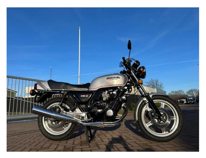
The 1978 Honda CBX1000Z is one of the most iconic motorcycles ever built, featuring a 1,047cc DOHC inline-six engine that set new standards in superbike performance. Known for its smooth power delivery, high-revving nature, and unmistakable exhaust note, the CBX1000Z remains one of the most desirable classics among collectors and enthusiasts.
